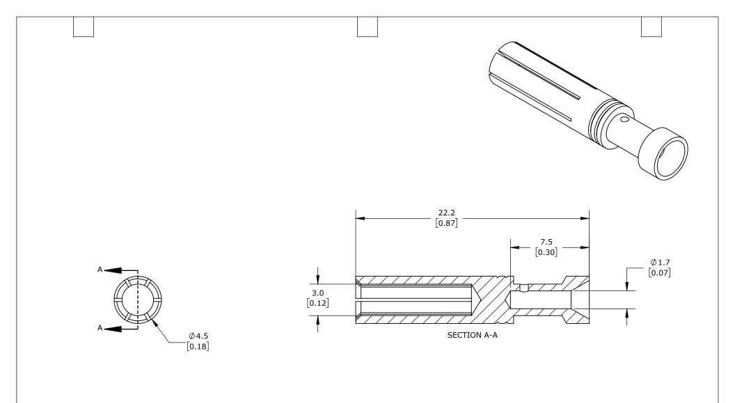
FEMALE, 16 AMP, ACCEPTS WIRE SIZE 16 AWG, SILVER-PLATED COPPER ALLOY. PACKAGE OF 100. FOR USE WITH METE MULTI-WIRE FEMALE INSERTS RATED FOR 16 AMPS.
