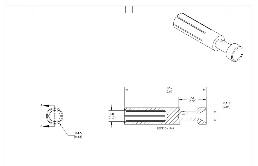
FEMALE, 16 AMP, ACCEPTS WIRE SIZE 20 AWG, SILVER-PLATED COPPER ALLOY. PACKAGE OF 100. FOR USE WITH METE MULTI-WIRE FEMALE INSERTS RATED FOR 16 AMPS.
