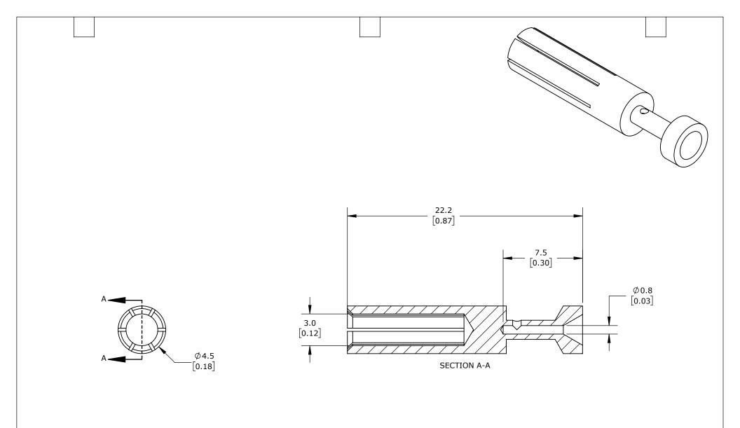
FEMALE, 16 AMP, ACCEPTS WIRE SIZE 26-22 AWG, SILVER-PLATED COPPER ALLOY. PACKAGE OF 100. FOR USE WITH METE MULTI-WIRE FEMALE INSERTS RATED FOR 16 AMPS.
