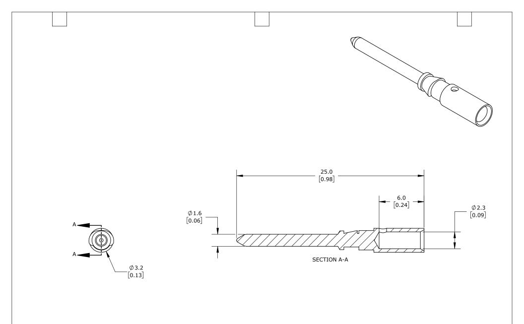
MALE, 10 AMP, ACCEPTS WIRE SIZE 14 AWG, SILVER-PLATED COPPER ALLOY. PACKAGE OF 100. FOR USE WITH METE MULTI-WIRE MALE INSERTS RATED FOR 10 AMPS.
