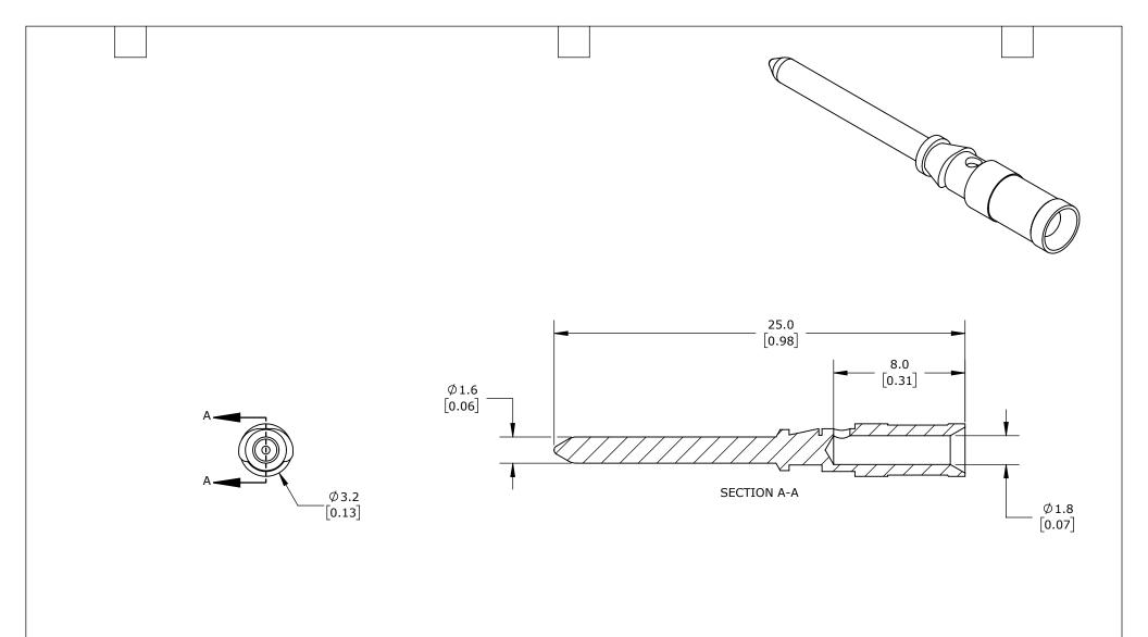
MALE, 10 AMP, ACCEPTS WIRE SIZE 16 AWG, SILVER-PLATED COPPER ALLOY. PACKAGE OF 100. FOR USE WITH METE MULTI-WIRE MALE INSERTS RATED FOR 10 AMPS.
