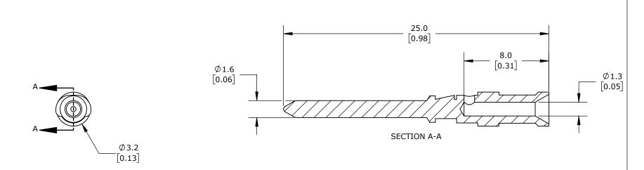
MALE, 10 AMP, ACCEPTS WIRE SIZE 18 AWG, SILVER-PLATED COPPER ALLOY. PACKAGE OF 100. FOR USE WITH METE MULTI-WIRE MALE INSERTS RATED FOR 10 AMPS.
