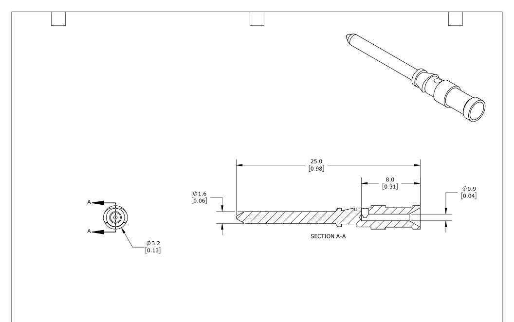
MALE, 10 AMP, ACCEPTS WIRE SIZE 26-22 AWG, SILVER-PLATED COPPER ALLOY. PACKAGE OF 100. FOR USE WITH METE MULTI-WIRE MALE INSERTS RATED FOR 10 AMPS.
