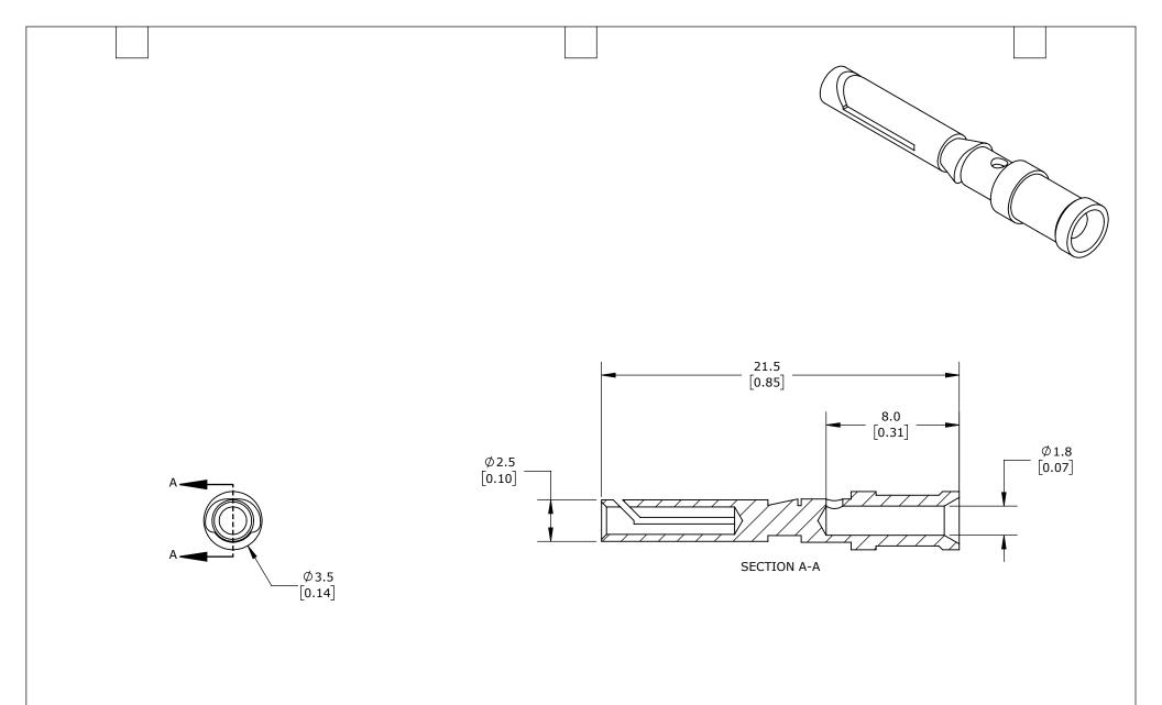
FEMALE, 10 AMP, ACCEPTS WIRE SIZE 16 AWG, SILVER-PLATED COPPER ALLOY. PACKAGE OF 100. FOR USE WITH METE MULTI-WIRE FEMALE INSERTS RATED FOR 10 AMPS.
