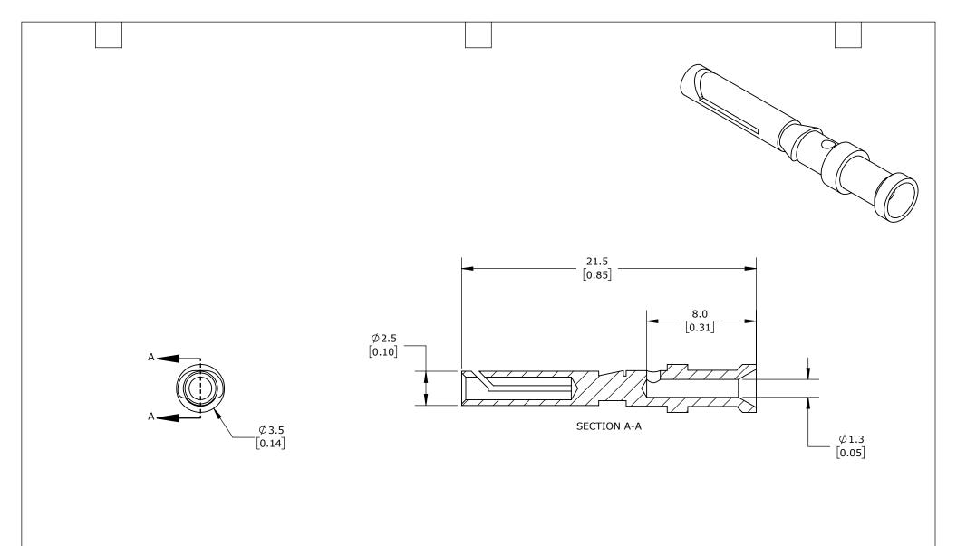
FEMALE, 10 AMP, ACCEPTS WIRE SIZE 18 AWG, SILVER-PLATED COPPER ALLOY. PACKAGE OF 100. FOR USE WITH METE MULTI-WIRE FEMALE INSERTS RATED FOR 10 AMPS.
