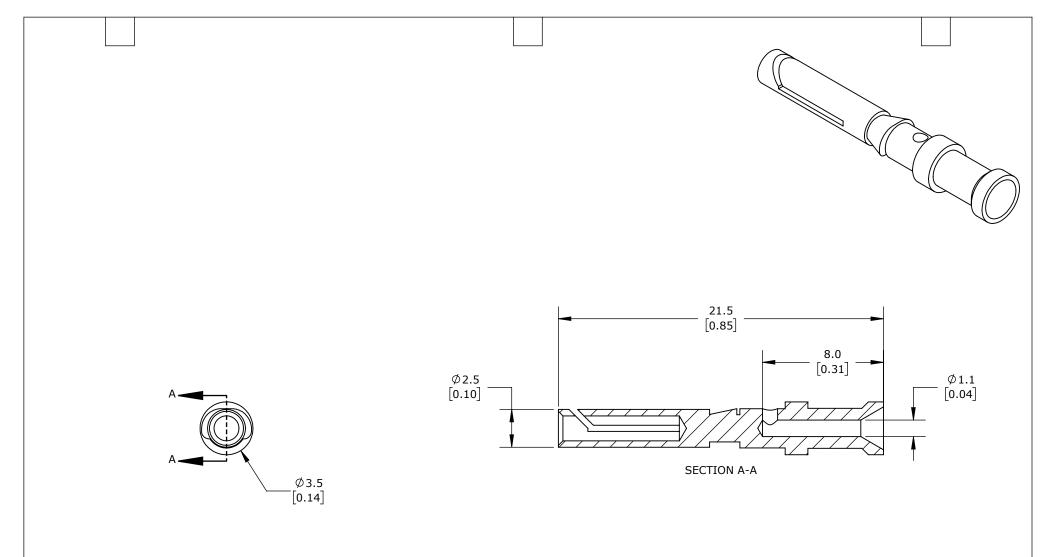
FEMALE, 10 AMP, ACCEPTS WIRE SIZE 20 AWG, SILVER-PLATED COPPER ALLOY. PACKAGE OF 100. FOR USE WITH METE MULTI-WIRE FEMALE INSERTS RATED FOR 10 AMPS.
