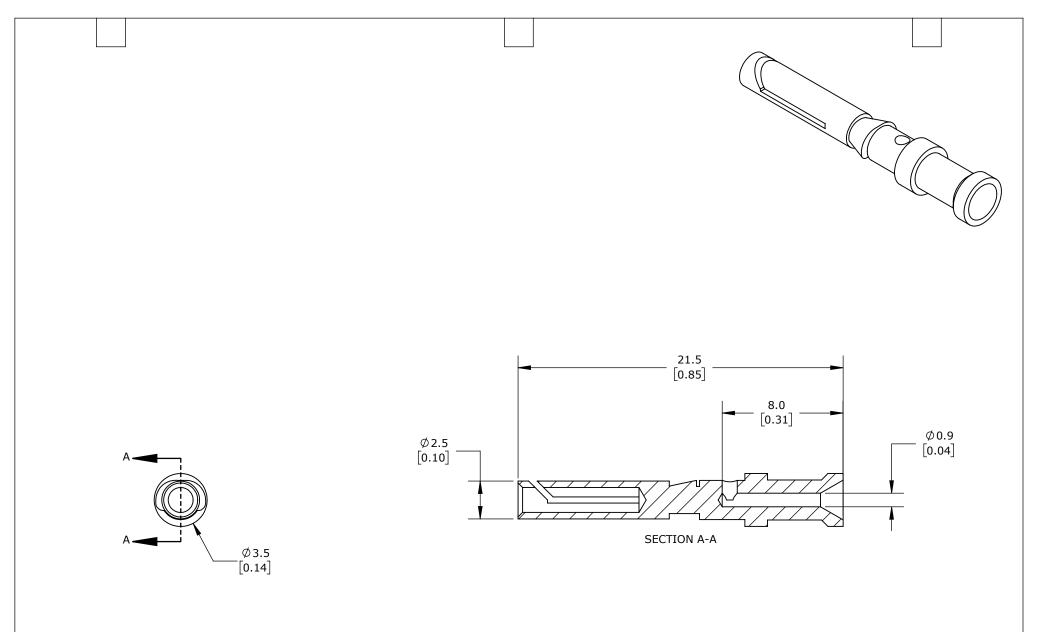
FEMALE, 10 AMP, ACCEPTS WIRE SIZE 26-22 AWG, SILVER-PLATED COPPER ALLOY. PACKAGE OF 100. FOR USE WITH METE MULTI-WIRE FEMALE INSERTS RATED FOR 10 AMPS.
