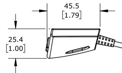
MANUAL SWITCH, IP30. FOR USE WITH ERGOSWISS 124.43800-PP000001 AND 124.43801-PP000001 CONTROL BOXES. (1) 6.5FT/2M POWER CABLE INCLUDED. SAVES (3) INTERMEDIATE POSITIONS IN ADDITION TO UP AND DOWN FUNCTION.
