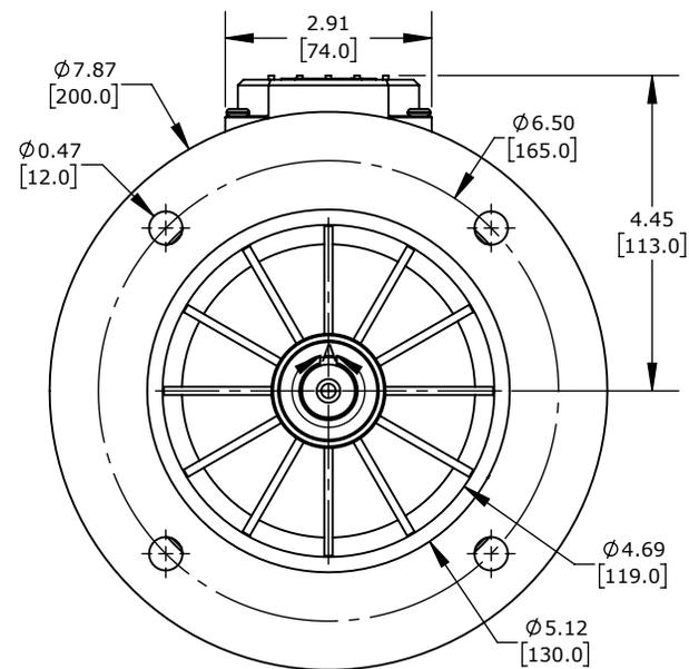
M.G.M. ELECTRIC MOTORS SMX IE3 PREMIUM EFFICIENCY AC INDUCTION MOTOR, GENERAL PURPOSE AND INVERTER RATED, 1HP, 3-PHASE, 230/460 VAC, 3600RPM, TEFC, IEC 80 FRAME, ALUMINUM, D-FLANGE (B5) MOUNT
