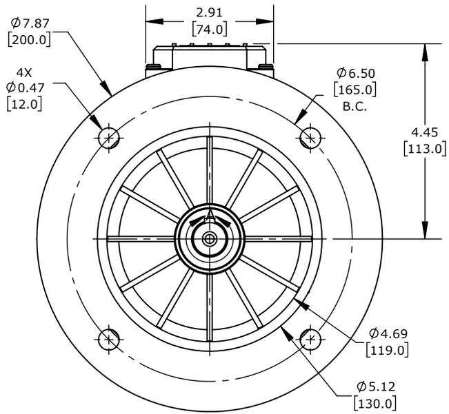
M.G.M. ELECTRIC MOTORS SMX IE3 PREMIUM EFFICIENCY AC INDUCTION MOTOR, GENERAL PURPOSE AND INVERTER RATED, 1HP, 3-PHASE, 230/460 VAC, 1800RPM, TEFC, IEC 80 FRAME, ALUMINUM, D-FLANGE (B5) MOUNT
