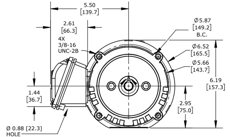
WEG ELECTRIC S SERIES STANDARD EFFICIENCY AC INDUCTION MOTOR, WITH BRAKE, GENERAL PURPOSE, INVERTER RATED, 1/2HP, 3-PH, 208-230/460 VAC, 1800RPM, TEFC, 56C FRAME, ROLLED STEEL, C-FACE ONLY MOUNT, STEARMS 105601100BQF BRAKE ASSEMBLY INCLUDED
