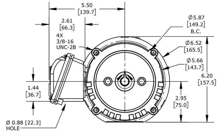
WEG ELECTRIC S SERIES STANDARD EFFICIENCY AC INDUCTION MOTOR, WITH BRAKE, GENERAL PURPOSE, INVERTER RATED, 1/3HP, 3-PH, 208-230/460 VAC, 1800RPM, TEFC, 56C FRAME, ROLLED STEEL, C-FACE ONLY MOUNT, STEARMS 105601100BQF BRAKE ASSEMBLY INCLUDED
