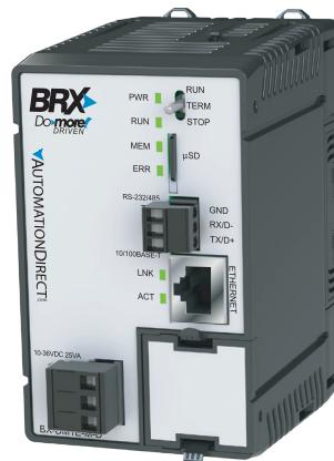
**BX-DM1E-M-D Micro PLC Unit (MPU)**
