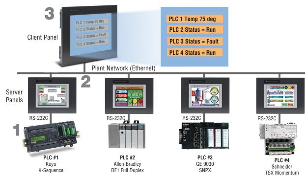
Each PLC is operating a seperate application and is connected to a **C-more** panel through a Serial Connection.
