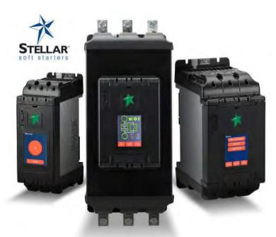
Soft starters are used to reduce the motor inrush current, along with moderating mechanical shock to the motor and downstream machinery. While soft starters are useful for all motor sizes, they are even more important for large motors, which would otherwise draw massive current if started across-the-line and potentially incur penalty demand charges from the electrical utility if the spikes occur at certain times of day.
