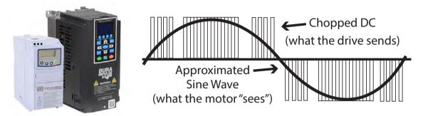
Basic VFD functions include overload protection, start/stop control, and adjustable acceleration/deceleration. Many other advanced capabilities are available, such as current limiting to reduce motor inrush current at startup, advanced control modes, additional input/output (I/O) connections, digital communications with supervisory systems, PID loop control, on-board programmable logic controller (PLC) control, and more.
