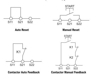
Note: A power supply unit with electrical isolation from the mains supply must be connected. External fusing of each safety output contact is necessary, a 4A slow-blow or 6A (quick action) must be provided. The maximum cabling and connecting resistance of control lines must not be exceed 300 Ohms.
