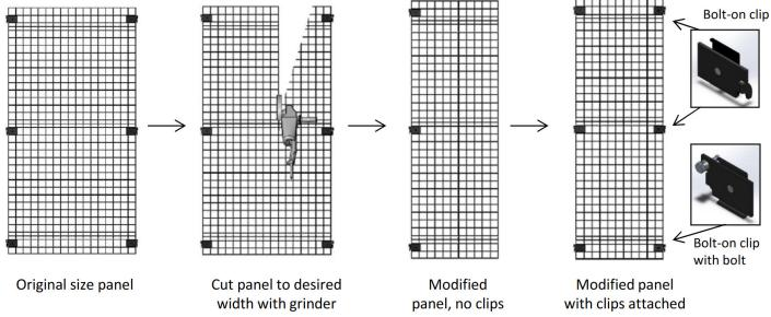
NOTE: When working on an 8ft high system, cut one side of the 66in high panel and the opposite side on the 24in.
