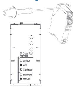
Disconnect unit before setting switches.
