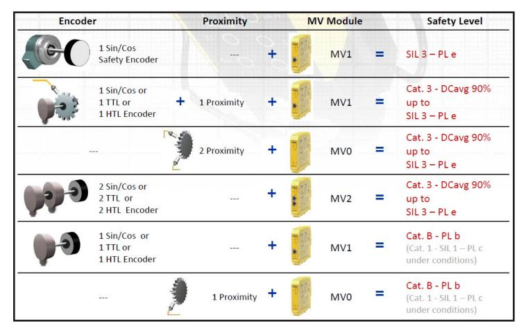
All MV Series Speed Monitor Expansion Units allow for up to 2 axes.
