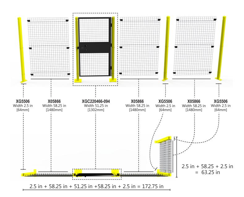
NOTE: The panels can be used as-is, or they can be field-cut to fit your particular installation needs. For example, a 58.25-inch-wide panel could be cut to a width of 54 in if that is what your installation requires. Please note that field-cut panels require additional mounting clips (sold separately).
