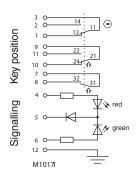
Fig. 2: Lock deactivated: Key removed
