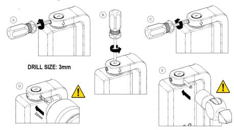
Installer MUST drill and pin switch in final switching position. Installer must not rely only on adjustment grub screw for safety. See operating instructions for additional information on switching angle window adjustment.
