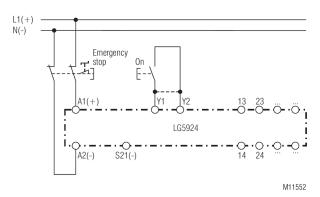
Two-channel emergency-stop circuit without feedback loop, with or without automatic restart. For automatic restart, terminals Y1-Y2 must be linked. No ON pushbutton necessary.
