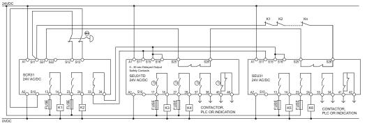
Dual channel, E-Stop, Auto reset with multiple expansion units
