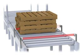
M5 photocells have five beams that are sent out by the emitter. If any one of the five beams is blocked, then the receiver's status signal will change to signify that there is an object in front of the photocell. This is particularly useful when there is a need to detect irregularly shaped items.
