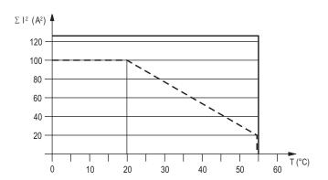
— AC / DC 24V device mounted on distance with air circulation. max. current at 55°C over
