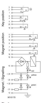
Solenoid locking deactivated: Magnet released, Key removed
