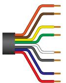
Orange – Guard open signal out Brown – Unlock signal +24VDC in
