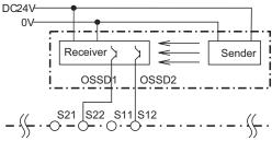
Fct.: Light curtain (8), without cross fault detection SIL 3, PL e, Cat. 4 <sup>2)</sup>
