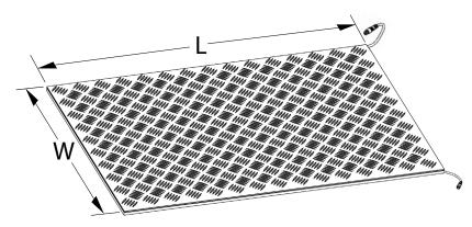
SENTIR safety contact mats are rectangular sections which are used to safeguard dangerous areas in industrial and production automation settings. Stepping on the mat triggers an immediate "stop" signal in order to prevent endangering movements.
