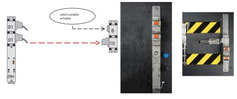
Keys trapped at main station (left). Door station with optional padlock module (right).
