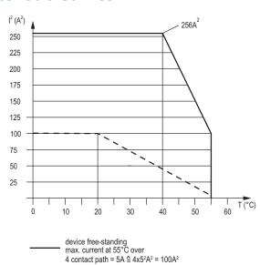
device mounted without distance heated by devices with same load, max. current at 55°C over
