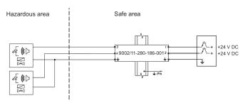
Application: Discrete 2-wire output for solenoid valves, LEDs and signalling devices
