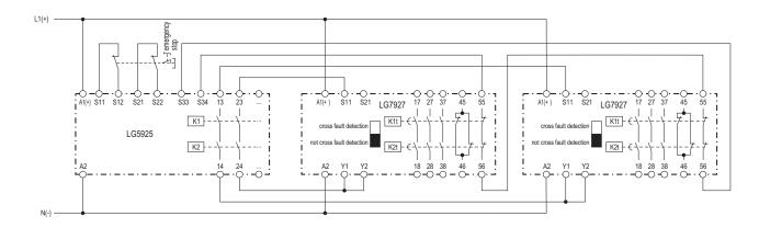
LG 5925 with two LG 7927, non cross fault detection, suitable up to SIL2, Performance Level d, Cat. 3
