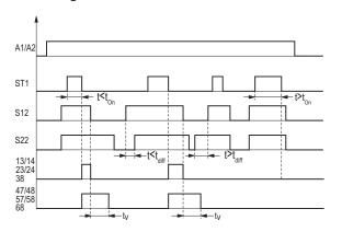
t ....: max. time delay for simultaneity demand dependent on selected safety function E-Stop, safety gate, safety mat t are: max. 3s Light curtains t<sub>diff</sub>: max. 1s Two-hand control t<sub>diff</sub>: max. 0,5s other times on request
