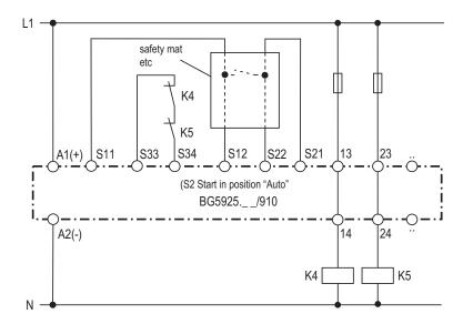
Switch gear for safety mats and edges
