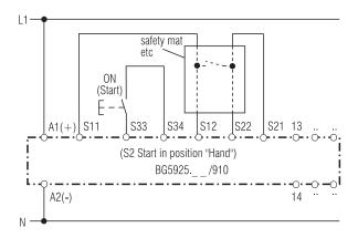
Switch gear for safety mats and edges switch S2 position: Manual start (For automatic restart S2 in position Autostart and link on S33-S34) Suited up to SIL3, Performance Level e, Cat. 4
