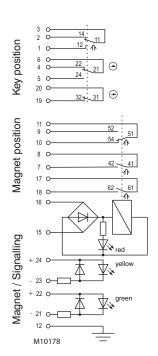
Solenoid locking deactivated: Magnet released, Key inserted
