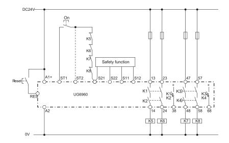
Safety function: see below, Manual-Start (for automatic start make a bridge to ST2 instead of ON button). Delay function: release delay (1)
