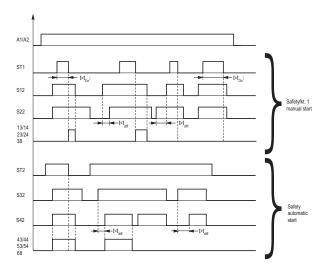
t<sub>air</sub> max. time delay for simultaneity demand dependent on selected safety function E-Stop, safety gate, safety mat t<sub>air</sub>: max. 3s Light curtains t<sub>air</sub>: max. 1s Two-hand control t<sub>air</sub>: max. 0,5s other times on request
