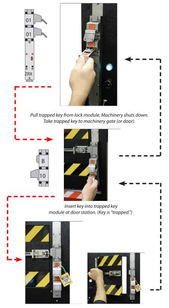
Remove (or optionally, lock out) optional safety key. (Access to machinery is unlocked. Enter machinery.)
