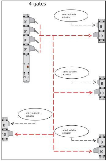
\*Suitable actuators: ST2317-T-ACTUATOR ST2311-C-ACTUATOR ST2312-CS-ACTUATOR
