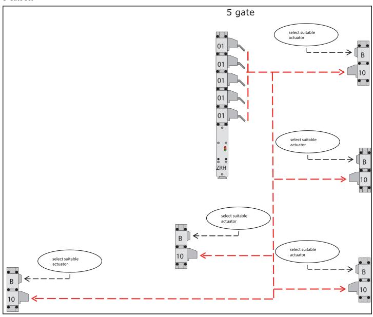
\*Suitable actuators: ST2317-T-ACTUATOR ST2311-C-ACTUATOR ST2312-CS-ACTUATOR
