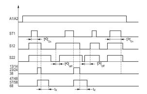
t .... max. time delay for simultaneity demand dependent on selected safety function E-Stop, safety gate, safety mat t :: max. 3s Light curtains t :: max. 1s Two-hand control t max. 0,5s other times on request
