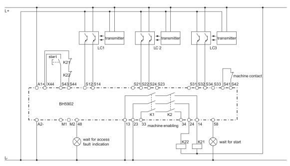
Stepping operation with 3 light curtains and contact reinforcement by external contactors, 2-channel operation (switching of feedback input can also be used at protective operation with muting)
