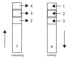
In the locking sequence, when each module is activated, it releases the module above it. Similarly, during the unlocking sequence, when a module is locked, it allows locking of the module below it.
