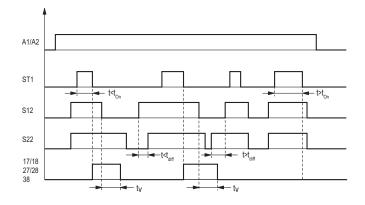
t,iff: max. time delay for simultaneity demand dependent on selected safety function E-Stop, safety gate, safety mat t<sub>niff</sub>: max. 3s Light curtains t<sub>diff</sub>: max. 1s Two-hand control t<sub>diff</sub>: max. 0,5s other times on request
