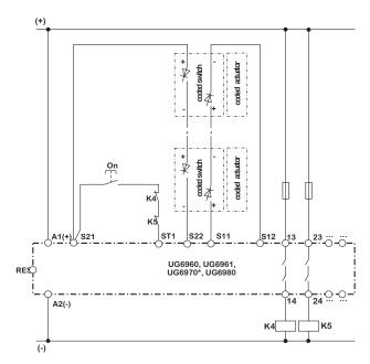
\*UG6970: The safety function 2 is connected as well as safety function 1, but S11'= S31, S12 = S32, S21 = S41, S22 = S42 and ST1 = ST2
