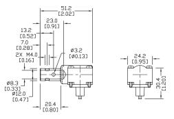
Figure 4: 90° adjustable head with lever hinge interlock - SP2K61, SDM2K61 models
