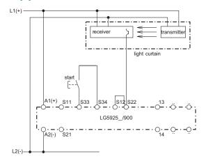
Single channel connection of light curtains with self-test according to EN 61 496-1.
