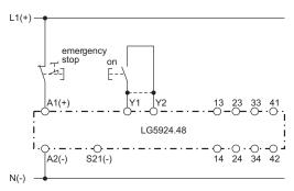
Single-channel, emergency-stop circuit without feedback loop, with or without automatic restart. For automatic restart, terminals Y1 - Y2 must be jumpered. No ON pushbutton necessary.
