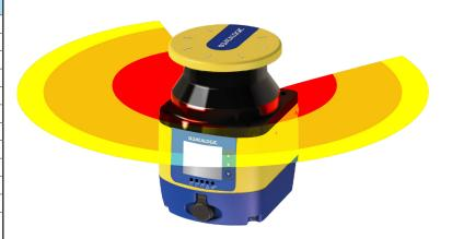
Datalogic Safety Laser Scanners can manage two simultaneous warning zones and one safe zone. Safe zones can extend up to 5.5 m [18.04 ft], depending on the model, over an angle of 275 degrees. Warning zones can extend 40m [131.2 ft].
