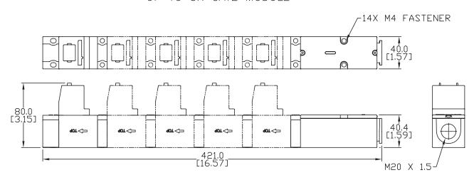
Note: SX-XGATE-SET also includes 1-5 GATE ACTUATOR MODULES, depending on the gate set kit number (1-5).
