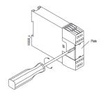
Disconnect unit before setting switches.
