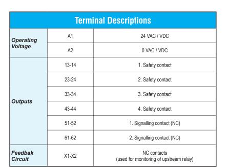
NOTE: Signalling contacts must not be used in safety circuits.
