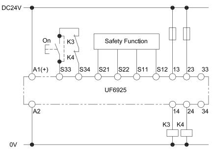
A jumper must be fitted at S33-S34 for the automatic ON function. The ON pushbutton is not required. The required start function has to be selected on switch S1 before starting the device. See "Unit Programming."
