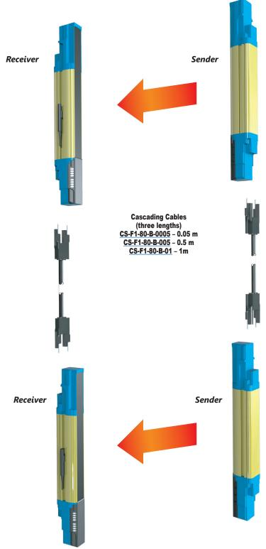
Note: A maximum number of three units, one master and two slaves, may be cascaded. The maximum length of the master unit is 1800mm and the maximum length of each slave is 1200mm.
