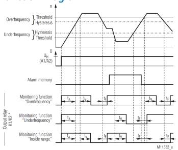
$t_A = Start$ -up delay,  $t_V = Alarm$  delay,  $t_F = Reset$  delay
