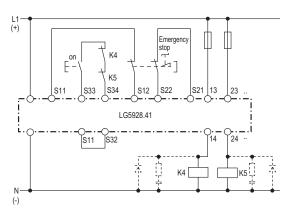
Contact reinforcement by external contactors, 2-channel controlled. The output contacts can be reinforced by external contactors with forcibly guided contacts for switching currents > 8 A e.g. 6 A.
