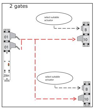
\*Suitable actuators: ST2317-T-ACTUATOR ST2311-C-ACTUATOR ST2312-CS-ACTUATOR
