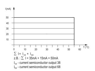
Quadratic total current limit curve semiconductor monitoring outputs
