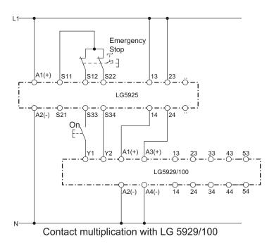
Note: This is a representative drawing. Depending on the LG5925 safety relay you select, different voltage sources may be required.
