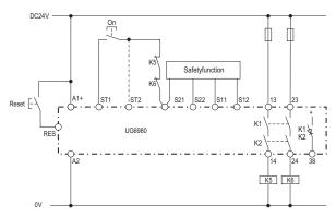
Safety function: see below, Manual-Start (for automatic start make a bridge to ST2 instead of ON button).
