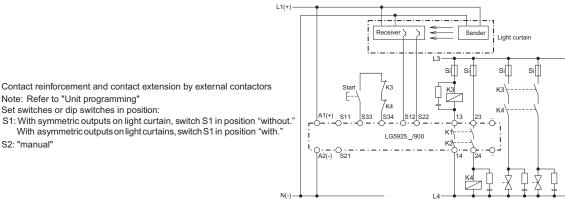
Contact reinforcement and contact extension by external contactors
