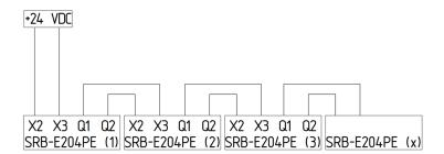
NOTE: While there is not a limit to the number of modules that can be wired in series, it is important to note that the response time of the system will change as more modules are added. For example, one unit will have a response time of less than 10ms. But if the user uses 10 modules in series (for a total of 40 inputs) then the response time of the system will be less than 100ms.
