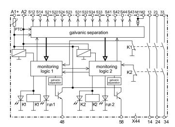
Note: All drawings are for a 3 N.O. configuration. The units will actually have a 2 N.O. and 1 N.C. configuration.
