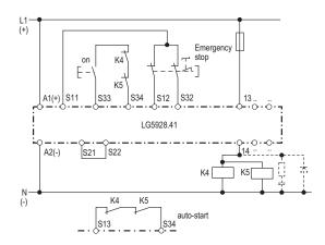
Contact reinforcement by external contactors controlled by one contact path. S33 - S34 must stay open on auto start.
