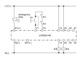
Contact reinforcement by external contactors, 2-channel controlled. For currents>5A, the output contacts can be reinforced by external contactors. Functioning of the external contactors is monitored by looping the N.C. contacts into the start circuit (Y1 - Y2).
