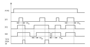
$t_{\mbox{\tiny diff}}$ : max. time delay for simultaneity demand dependent on selected safety function E-Stop, safety gate, safety mat t<sub>eff</sub>: max. 3s Light curtains  $t_{\text{diff}}$ : max. 1s Two-hand control  $t_{\text{diff}}$ : max. 0,5s other times on request
