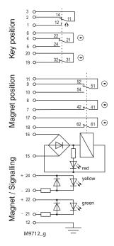
Solenoid locking activated: Magnet locked, Key inserted
