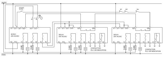
Dual channel, E-Stop, Manual reset with multiple expansion units
