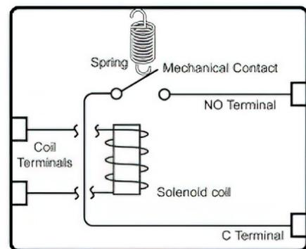
Electro-mechanical relays use a small electrical control signal to shift contacts operating a separate circuit. The spring opposes the electro-mechanical action and returns the contact to its rest state when the coil is de-energized.
