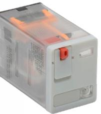
**Force guided relays** provide fail-safe operation by mechanically linking the N.O. and the associated N.C. contact. This ensures that one contact is closed while the other is open, preventing damage to equipment.
