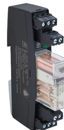
**Force guided relays** provide fail-safe operation by mechanically linking the N.O. and the associated N.C. contact. This ensures that one contact is closed while the other is open, preventing damage to equipment.
