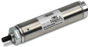
NITRA pneumatic stainless steel round body, interchangeable, non-repairable cylinder, 1-1/16 inch bore, 1/8 NPT port, single acting, spring return, front nose mount.
