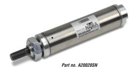
NITRA pneumatic stainless steel round body interchangeable, non-repairable cylinder, 1-1/4 inch bore, 1/8 NPT port, single acting, spring return, front nose mount.
