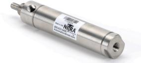
NITRA pneumatic stainless steel round body, interchangeable, non-repairable cylinder, 1-1/16 inch bore, 1/8 inch female NPT ports, double acting, front nose mount.
