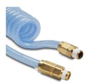
NITRA<sup>™</sup> reinforced coiled hose has a sturdy polyester braid between the polyurethane inner and outer layers. Contamination of air systems caused by rubber hose breakown is significantly reduced by using NITRA PUR hose. Standard hoses have one rigid and one swivel fitting and are specified by inside diameter. QC hoses have one Male and one Female industrial interchange quick disconnect fitting.
