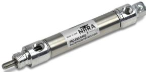
NITRA pneumatic stainless steel round body, interchangeable, non-repairable cylinder, 3/4 inch bore, 1/8 NPT ports, double acting, rear pivot mount (pivot pin included), magnetic piston.
