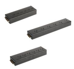
NITRA pneumatic control distribution blocks are a convenient way to connect a bank of valves to a controller. Replace all the wiring connectors supplied with the solenoid valves with this distribution block, and replace a bundle of solenoid cables with one DB15 cable. Each block matches up with a manifold of two to eight stations and includes built-in surge suppression and LED indication.
