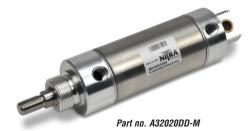
NITRA pneumatic stainless steel round body, interchangeable, non-repairable cylinder, 2 inch bore, 1/4 NPT ports, double acting, double end mount, magnetic piston.
