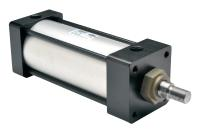
NITRA heavy duty pneumatic, NFPA interchangeable cylinder, 3-1/4 inch bore, 1 inch diameter piston rod, 1/2" female NPT ports, double acting, tapped end caps and one side for mount, flange, pivot and clevis mount options available. Some models available with cushions on both ends.
