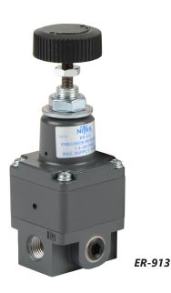
NITRA<sup>®</sup> ER Series Precision Regulators are miniature regulators that are designed to provide the highest level of regulation accuracy and repeatability available in a compact, lightweight housing. A force balanced pilot control maintains output pressure to within 0.05 psig (3.44 millibar) with minimal drift over time. They are ideal for applications that require exact pressure control and substantial flow capacity under variable operating conditions with limited space.
