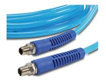
NITRA<sup>™</sup> reinforced polyurethane (PUR) hose features a sturdy polyester braid between the polyurethane inner and outer layers. Contamination of air systems caused by rubber hose breakdown is significantly reduced by using NITRA PUR hose. CBL2 and CBL3 hoses have one rigid and one swivel fitting and are specified by inside diameter. CBL5 and CBL6 hoses have one Male and one Female industrial interchange quick disconnect fitting.
