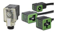
These high quality connectors and over-molded cables help reduce wiring time. The lower voltage models, 24V or 110V AC/DC, include built-in surge suppression, Yellow LED indicator and are rated for connecting with electronics. The 230V AC/DC models are rated for straight wired products. All models are available in five sizes based on DIN 43650.
