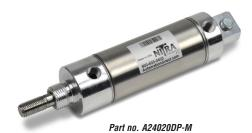
NITRA pneumatic stainless steel round body, interchangeable, non-repairable cylinder, 1-1/2 inch bore, 1/8 NPT ports, double acting, rear pivot mount, magnetic piston (pivot pin included). Cylinder cannot be double end mounted.
