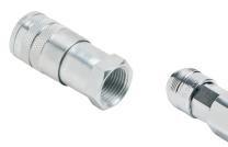
**NITRA** pneumatic quick-disconnect hose couplings allow easy changing of tools or hose connections. Couplers and plugs are sold separately. Industrial Interchange, ARO210 and Truflate plugs are available in steel and chrome-plated steel. Couplers are available in Industrial Interchange manual or automatic and universal automatic. Safety couplers bleed off air pressure downstream before disconnecting.
