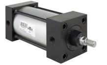
NITRA heavy duty pneumatic, NFPA interchangeable cylinder, 2-1/2" bore, 5/8" diameter piston rod, 7/16"-20 male threaded end, 1/4" female NPT ports, double acting, tapped end caps and one side for mount, flange, pivot and clevis mount options available. Some models available with cushions on both ends.
