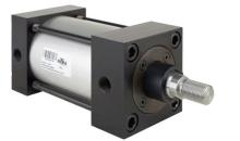
NITRA heavy duty pneumatic, NFPA interchangeable cylinder, 3-1/4" bore, 1" diameter piston rod, 3/4"-16 male threaded end, 3/8" female NPT ports, double acting, tapped end caps and one side for mount, flange, pivot and clevis mount options available. Some models available with cushions on both ends.
