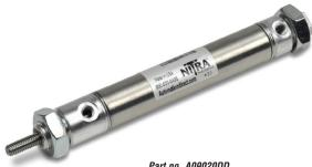
NITRA pneumatic stainless steel round body, interchangeable, non-repairable cylinder, 9/16 inch bore, #10-32 ports, double acting, double end mount.
