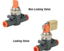
**NITRA** pneumatic push-to-connect in-line hand valves have a technopolymer body and nickel-plated brass valve insert, with a range of 0 to 150 psi. Both 2-way and 3-way valves are available with or without locking capability. 3-way valves relieve pressure downstream when in the closed position.
