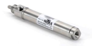
NITRA pneumatic stainless steel round body, interchangeable, non-repairable cylinder, 3/4 inch bore, 1/8 inch female NPT ports, double acting, front nose mount.
