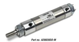
NITRA pneumatic stainless steel round body interchangeable, non-repairable cylinder, 1-1/4 inch bore, 1/8 NPT ports, double acting, double end mount, magnetic piston.
