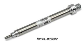
NITRA pneumatic stainless steel round body, interchangeable, non-repairable cylinder, 7/16 inch bore, #10-32 port, single acting, spring return, rear pivot mount (pivot pin included).
