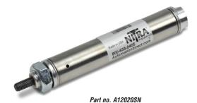
NITRA pneumatic stainless steel round body, interchangeable, non-repairable cylinder, 3/4 inch bore, 1/8 NPT port, single acting, spring return, front nose mount.
