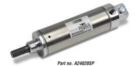
**NITRA** pneumatic stainless steel round body, interchangeable, non-repairable cylinder, 1-1/2 inch bore, 1/8 NPT port, single acting, spring return, rear pivot mount (pivot pin included). Cylinder cannot be double end mounted.
