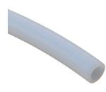
**NITRA** PTFE tubing is made from the highest quality, 100% virgin raw materials and has a hardness specification of Shore D 55. PTFE tubing is an excellent choice for many high heat applications. It has exceptional resistance to degradation of mechanical properties under severe conditions. NITRA PTFE tubing does not support combustion and has very good dielectric properties. **NITRA** PTFE is ideal for use with **NITRA** stainless steelpushto-connect fittings.
