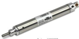
NITRA pneumatic stainless steel round body, interchangeable, non-repairable cylinder, 9/16 inch bore, #10-32 port, single acting, spring return, double end mount.
