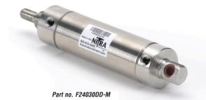
NITRA pneumatic stainless steel round body, interchangeable, non-repairable cylinder, 1-1/2 inch bore, 1/8 inch female NPT ports, double acting, double end mount, magnetic piston.
