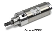
NITRA pneumatic stainless steel round body, interchangeable, non-repairable cylinder, 2 inch bore, 1/4 NPT ports, double acting, front nose mount.
