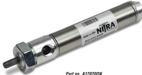
NITRA pneumatic stainless steel round body, interchangeable, non-repairable cylinder, 3/4 inch bore, 1/8 NPT ports, double acting, front nose mount.
