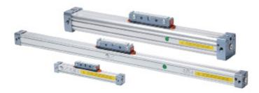
NITRA L-Series Rodless Cylinders offer a robust design in a compact package. Rodless cylinders can offer the same stroke as rodded cylinders in a smaller space. All sizes have magnetic pistons and are double acting. Mounting brackets and cylinder position switches are sold separately.
