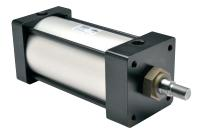
**NITRA** heavy duty pneumatic, NFPA interchangeable cylinder, 4 inch bore, 1 inch diameter piston rod, 1/2" female NPT ports, double acting, tapped end caps and one side for mount, flange, pivot and clevis mount options available. Some models available with cushions on both ends.
