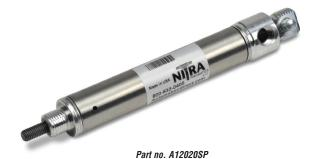
NITRA pneumatic stainless steel round body, interchangeable, non-repairable cylinder, 3/4 inch bore, 1/8 NPT port, single acting, spring return, rear pivot mount (pivot pin included).
