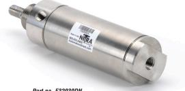
NITRA pneumatic stainless steel round body, interchangeable, non-repairable cylinder, 2 inch bore, 1/4 inch female NPT ports, double acting, front nose mount.
