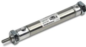
NITRA pneumatic stainless steel round body, interchangeable, non-repairable cylinder, 9/16 inch bore, #10-32 ports, double acting, double end mount, magnetic piston.
