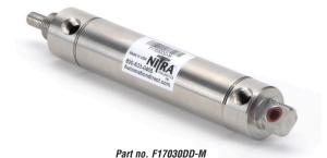
NITRA pneumatic stainless steel round body, interchangeable, non-repairable cylinder, 1-1/16 inch bore, 1/8 inche female NPT ports, double acting, double end mount, magnetic piston.
