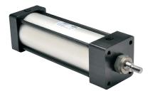
**NITRA** heavy duty pneumatic, NFPA interchangeable cylinder, 2-1/2 inch bore, 5/8" diameter piston rod, 1/4" female NPT ports, double acting, tapped end caps and one side for mount, flange, pivot and clevis mount options available. Some models available with cushions on both ends.
