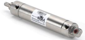
**NITRA** pneumatic stainless steel round body, interchangeable, non-repairable cylinder, 1-1/16 inch bore, 1/8 inch female NPT ports, double acting, double end mount.
