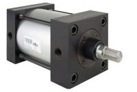
NITRA heavy duty pneumatic, NFPA interchangeable cylinder, 4" bore, 1" diameter piston rod, 3/4"-16 male threaded end, 3/8" female NPT ports, double acting, tapped end caps and one side for mount, flange, pivot and clevis mount options available. Some models available with cushions on both ends.
