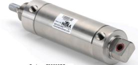
**NITRA** pneumatic stainless steel round body, interchangeable, non-repairable cylinder, 2 inch bore, 1/4 inch female NPT ports, double acting, double end mount.
