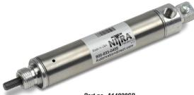
NITRA pneumatic stainless steel round body, interchangeable, non-repairable cylinder, 7/8 inch bore, 1/8 NPT port, single acting, spring return, rear pivot mount (pivot pin included).
