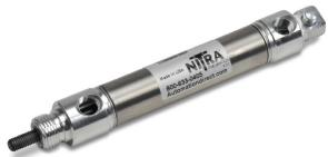
NITRA pneumatic stainless steel round body, interchangeable, non-repairable cylinder, 3/4 inch bore, 1/8 NPT ports, double acting, rear pivot mount (pivot pin included).
