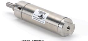
NITRA pneumatic stainless steel round body, interchangeable, non-repairable cylinder, 1-1/2 inch bore, 1/8 inch female NPT ports, double acting, front nose mount.
