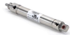
NITRA pneumatic stainless steel round body, interchangeable, non-repairable cylinder, 3/4 inch bore, 1/8 inch female NPT ports, double acting, double end mount.
