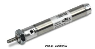
NITRA pneumatic stainless steel round body, interchangeable, non-repairable cylinder, 9/16 inch bore, #10-32 ports, double acting, front nose mount.
