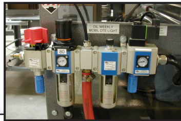
Air preparation system (shut-off/lock-out, combination filter/regulator, soft start valve, lubricator if needed)
