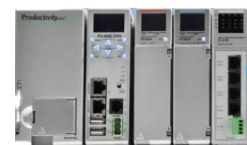
PLC Sends commands and status requests via EtherNet/IP
