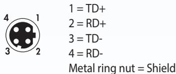
OUT or P2 (M12 female connector, D encoding)
