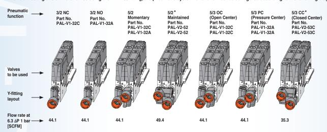
In order to get 5/2 momentary, 5/2 maintained and 5/3 CC high flow, use two parallel valves, by energizing the solenoids simultaneously.
