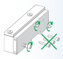
Note: Version used to make up a PAL Base without pneumatic valves, but only with "S" signal modules and fieldbus or additional electrical connection "E". Pneumatic bases and valves cannot be added.
