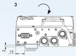
Mounting with brackets: The 3 brackets are included with each PAL stand-alone valve base. Push them firmly into the appropriate seats on the bases until they "click".
