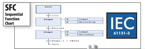
For those unfamiliar with CODESYS, this software package was first developed by 3S-Smart Software Solutions in 1994. Since then, it has become the most widely used manufacturer independent IEC 61131-3 development system in the world. CODESYS is used in all sectors of the automation industry and in a wide variety of applications. OEMs, end users, system integrators, and more have found CODESYS to be a powerful, versatile solution for their project needs.
