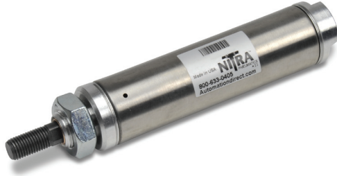
Cylinder, 1-1/4 in bore, single acting, spring return, front nose mount
