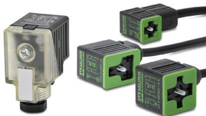
These high quality connectors and over-molded cables help reduce wiring time. The lower voltage models, 24 V or 110 V AC/DC, include built-in surge suppression, Yellow LED indicator and are rated for connecting with electronics. The 230 V AC/DC models are rated for straight wired products. All models are available in five sizes based on DIN 43650.
