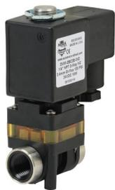
The Nitra DVM-2B Series valves are media separated, dry operator, 2-way, 2-position solenoid operated valves for use with gases or fluids where the metal working components of the valves do not come into contact with the working fluid. Three orifice
