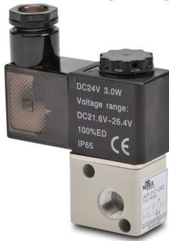
NITRA™ pneumatic AVP series directional control solenoid valves are 3-way stackable poppet style valves with 1/8" NPT ports. They provide 2-position, normally closed, spring return operation with either 24 VDC or 120 VAC solenoid coils. The AVP series can be used in individual valve applications or multiple valves can be field assembled (stacked) to share supply air, simplifying piping connections. The DIN style wiring connector includes LED indication of the solenoid coil status.
