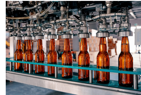
Food and beverage processing, such as this bottling line are great applications to use NEMA 4X drive as they require regular washdowns
