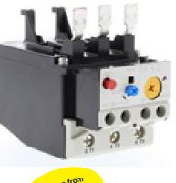
Fuji Electric Duo series TK-E overload relays protect motor windings from burning due to overloads, locked rotor current, or open phases. They are available in 5 different frame widths and are designed to directly mount to Fuji Electric Duo SC-E02P(G) through SC-E7 series IEC contactors. Optional mounting brackets allow the overloads to be separately DIN rail or panel mounted.
