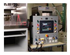
The completed system allows users to quickly connect the heater to be tested, enter test parameters, and run the test. Trend charts on the C-more panel track test parameters and quickly identify potential issues such as sudden drops in current or temperature.
