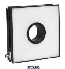
WenglorTPL Vision's Flat Dome Light is a high-power flat dome illumination solution for machine vision applications such as Pick and Place or Logistics. The LEDs are mounted with highly efficient lenses, engineered to distribute the highest brightness and uniformity balance available for machine vision applications.
