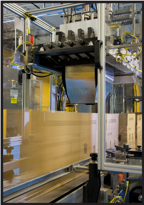
A packaging machine using T-slotted aluminum rail as an enclosure around the working parts of the machinery
