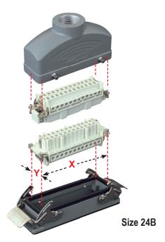
The size of each type of connector is determined by the distance between the center points of the four installation screws. These four points are common to both the insert and the housing. This is indicated by "X"-"Y" in the illustration above.
