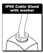
For securing a cable to the housing. This gland is available in plastic or metal in relation to housing material. Includes two washers and four gaskets to accommodate a wide range of cable diameters.
