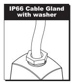
For securing a cable to the housing. This gland is available in plastic or metal in relation to housing material. Includes two washers and four gaskets to accommodate a wide range of cable diameters.
