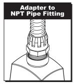
This adapter converts the Pg thread to an NPT thread. Sizes range from 3/8" to 1-1/4" in relation to the Pg threaded opening in the housing.
