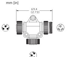
Note: Tightening torque 44 lb in (5.0 N·m) coupling nut.
