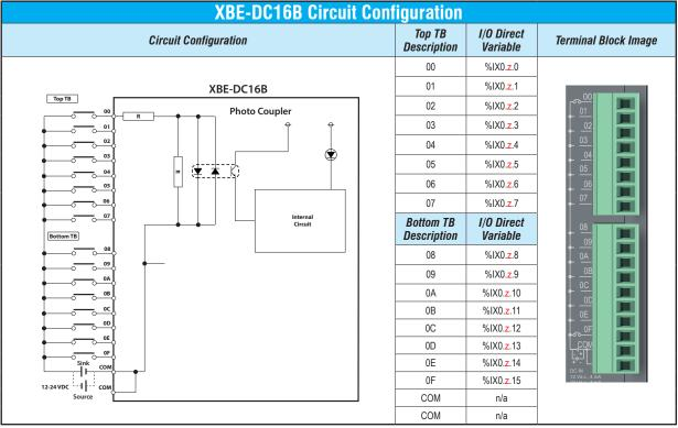
Note: Can be wired sinking or sourcing. In the I/O Direct Variable name, z=slot number.
