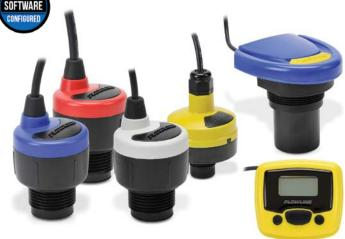
The EchoPod and EchoSonic II are innovative ultrasonic liquid level sensor families that replace float, conductance and pressure sensors that fail due to contact with dirty, sticky and scaling media in small, medium and large capacity tanks. Applied in chemical, water and wastewater applications, these general purpose non-contact sensors are available with single and multi-function capabilities including continuous level measurement, switching and control.
