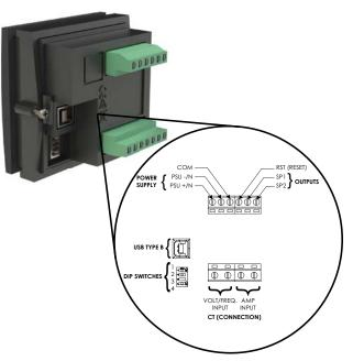
**Note:** DIP switch setting is 0 for positions 1, 2, 3 and 4 off. To change the default setting, visit <u>https://support.automationdirect.com/down-loads.html#tools</u> for free Trumeter ADM configuration utility download.
