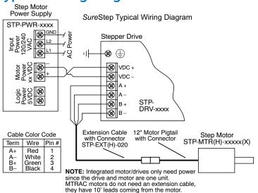
NOTE: STP-MTRAC-23xxx/34xxx motors and STP-DRVAC drives are designed to work with AC input power to the drive. They are not designed to work with DC input power.
