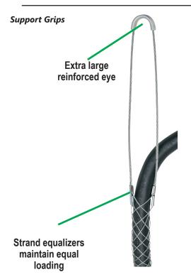
Support Grips are applied to the vertical or horizontal runs of cable or service lines to support dead weight and reduce potential damage due to breakage or stress. These grips are designed to be used indoors for cable support where flexible cable connects electrical equipment to bus duct. Applications also include support for air hoses and water hoses.
