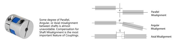
(Refer to the specification tables herein for the particular specifications of each type of drive coupling.)
