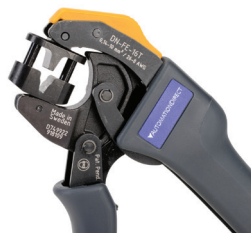
DN-FE-16T in Side Crimp Setting
