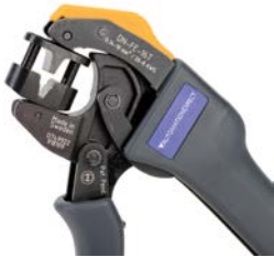
DN-FE-16T in Side Crimp Setting
