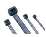
These ties are fabricated with a special composite of 6.6 polyamide and metal powder and are sensitive to electromagnetic fields. They are recommended in the food, pharmaceutical and chemical industry. They are useful in applications where, for safety reasons, it is necessary for a metal detector to be able to detect even very small fragments of these ties that may be mixed in with products.
