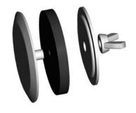
Extra pushbutton holes can be sealed against dust, dirt, oil, and water with a SCE hole seal. Seals will cover most pushbutton hole sizes. Hole seals come with oil-resistant gasket,  $\#10-32 \times 3/8$ ″ stud, zinc plated wing nut, and plated steel back plate. Available in stainless steel or powder coated finish.
