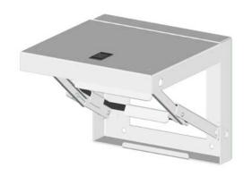
Folding shelves can be installed on the inside or outside of large enclosures. They are designed to support test and programming equipment. Locks in the horizontal position. When not in use, shelf can be folded down. Made of heavy gauge steel and powder coated. "SS" parts are stainless steel type 304 with a #4 brush finish. Provided with cULus Recognized sealing washer to maintain environmental rating of the enclosure.
