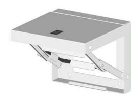
Folding shelves can be installed on the inside or outside of large enclosures. They are designed to support test and programming equipment. Locks in the horizontal position. When not in use, shelf can be folded down. Made of heavy gauge steel and powder coated. "SS" parts are stainless steel type 304 with a #4 brush finish. Provided with cULus Recognized sealing washer to maintain environmental rating of the enclosure.
