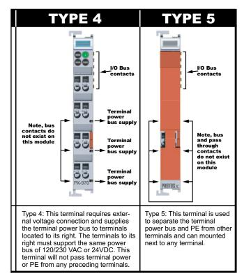
www.automationdirect.com Universal Field I/O tFED-26
